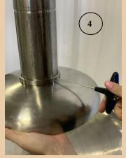
**Step 5**: Place the third tier over the cylinder, allowing it to rest on the tier below. Then place the crown on top of the cylinder. Finally, raise the third tier until it butts up against the bottom of the crown and tighten the set screws. There is no placement groove for this tier. (Note: Do not insert the auger until Step 9 after you have melted your chocolate.)
