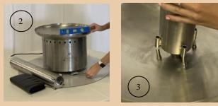
**Step 3**: Place the cylinder on the four prongs in the center of the basin so that it stands in place.
